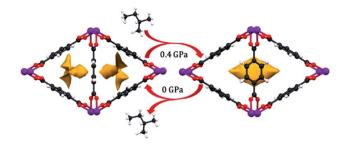
Fig. 9 Pore shape modification of Sc<sub>2</sub>BDC<sub>3</sub> upon exposure to 2methylbutane at elevated pressure. Rotation of the phenyl rings reveals a larger cavity that can accommodate molecules that cannot fit in the pores at ambient conditions. Reprinted with permission from ref. 77. Copyright 2015, American Chemical Society
