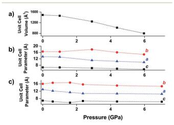
Fig. 6 (a) Unit cell volume of MIL-53(Al), (b) unit cell parameters of MIL-53(Al), and (c) unit cell parameters of NH<sub>2</sub>-MIL-53(Al) as a function of pressure. The parameter corresponding to the b-axis exhibits a notable increase at low pressures—an example of negative linear compression. Adapted from ref. 54 – published by the Royal Society of Chemistry.
