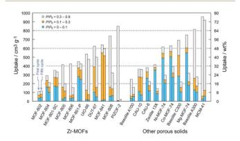
Fig. 10 Water uptake capacity of Zr-based MOFs (left) and other representative porous solids (right) in different pressure ranges (asterisk (\*) indicates no data). Left and right bars represent the first and fifth cycles, respectively. For MOF-801-SC (SC = single crystal form), uptake capacities of the first and second cycles were demonstrated. Reproduced from ref. 169 with permission from the American Chemical Society, copyright 2014.
