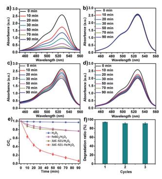
Fig. 4 UV-vis spectra of Rh6G agueous solution in the presence of JUC-521-Fe/H<sub>2</sub>O<sub>2</sub> (a), H<sub>2</sub>O<sub>2</sub> (b), FeSO<sub>4</sub>/H<sub>2</sub>O<sub>2</sub> (c) and JUC-521/H<sub>2</sub>O<sub>2</sub>(d). (e) Comparison of the degradation abilities of Rh6G for different materials. (f) Recyclability study of JUC-521-Fe
