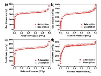
Fig. 3 N<sub>2</sub> adsorption-desorption isotherms of JUC-520 (a), JUC-521 (b), JUC-522 (c), and JUC-523 (d).
