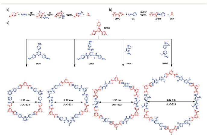
Scheme 1 Strategy for ambient aqueous-phase synthesis of COFs. (a) Mechanistic pathway of the Michael addition–elimination reaction of  $\beta$ -ketoenamines and aromatic amines. (b) Model reaction between DPPO and BA to form APPO and DMA. (c) Condensation of TDOEB and TAPT, TCTAB, DMB or DMOB to give JUC-520, JUC-521, JUC-522 or JUC-523 with different pores.
