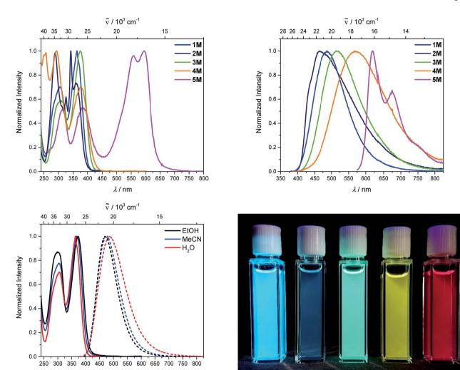
Fig. 3 Absorption (top, left) and emission spectra (top, right) of 1M-5M in water. Compound 2M was dissolved in 10% MeCN in water. Absorption and emission spectra of 1M in various solvents (EtOH: black, MeCN: blue,  $H_2O$ : red) (bottom, left) and picture of the solutions of 1M-5M in MeCN under UV irradiation.
