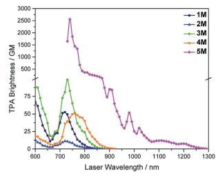
Fig. 7 Two-photon absorption spectra (left) and two-photon brightness ( $\sigma_2 \Phi_f$ ) (right) of 1M-5M in MeCN.
