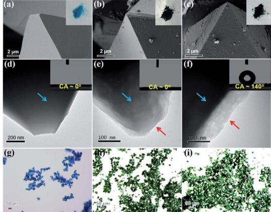
Fig. 2 SEM, TEM and light microscope images of HKUST-1 (a, d, g), HKUST-1@PDA (b, e, h) and HKUST-1@PDA-SF (c, f, i). The insets are the photograph and water contact angle (CA) of the corresponding samples. TEM images show that the MOF (blue arrow) are coated with a uniform polymer layer (red arrow).
