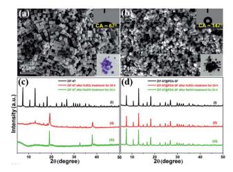
Fig. 5 SEM images of ZIF-67 nanocubes (a), hydrophobically modified ZIF-67@PDA-SF (b), and XRD patterns of ZIF-67 and ZIF-67@PDA-SF after exposure to  $\rm H_2SO_4$  (pH = 3)/NaOH (pH = 13) solution for 24 h (c and d). The insets are the water contact angles (CA) and a photograph of ZIF-67 (a) and ZIF-67@PDA-SF (b), respectively.
