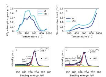
Fig. 4 TPD spectra for N0 and N50: (a)  $\rm CO_2$  desorption rates from TPD, (b) CO desorption from TPD, XPS spectra for N0 and N50: (c) N0 and (d) N50.
