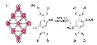
Fig. 8 (a) Crystal structure of UiO-66. (b) Scheme of the post-synthetic modification of UiO-66(SH) $_2$  to introduce sulfonic acid groups.
