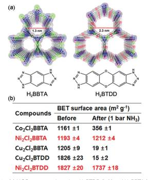
Fig. 13 (a) MOF structures based on  $\rm H_2BTDD$  (left) and  $\rm H_2BBTA$  (right) ligands. (b) Brunauer–Emmett–Teller (BET) surface area change after NH $_3$  exposure. Reproduced from ref. 66 with permission from American Chemical Society, Copyright 2018.
