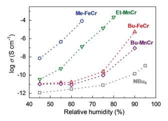
Fig. 6 Humidity dependence of the proton conductivity at 298 K. The blue, green, red, purple, and gray colors correspond to the proton conductivity of Me–FeCr, Et–MnCr, Bu–FeCr, Bu–MnCr, and NBu<sub>4</sub>, respectively. Reproduced from ref. 49 with permission from American Chemical Society, Copyright 2012.
