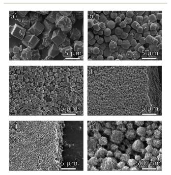
Fig. 5 SEM images of polyIRMOF-1 prepared from polymer ligands: (a) pbdc-8a; (b) pbdc-8a-PEG $_{2000}$ -2%; (c) pbdc-8a-PEG $_{4000}$ -1%; (d) pbdc-8a-PEG $_{2000}$ -20%; (e and f) pbdc-8a-PEG $_{4000}$ -10%.
