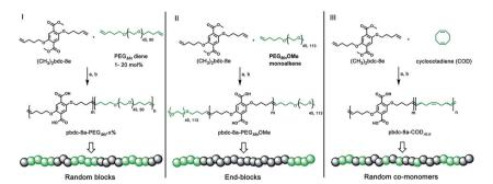
Scheme 1 Synthesis of three types of polymer ligands used in this work: (i) random AB PEG block copolymer ligand (pbdc-8a-PEG<sub> $M_n$ </sub>-x%); (ii) capped AB<sub>2</sub> PEG block copolymer ligand (pbdc-8a-PEG<sub> $M_n$ </sub>OMe); (iii) random AB COD block copolymer ligand (pbdc-8a-COD<sub>m:n</sub>). Reagents and conditions: (a) G2 catalyst, CH<sub>2</sub>Cl<sub>2</sub>, 50 °C, 5 h; (b) KOH, THF/H<sub>2</sub>O, 40 °C, 12 h.
