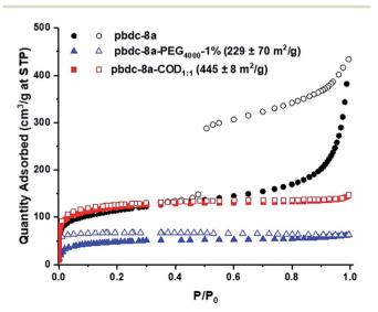
Fig. 4 Representative  $N_2$  isotherms of block-polyUiO-66 prepared from various block copolymer ligands that result in intergrown octahedra. The BET surface areas are included in parentheses. polyUiO-66 prepared from homopolymer pbdc-8a is included for comparison. Closed and open symbols represent the adsorption and desorption processes, respectively.
