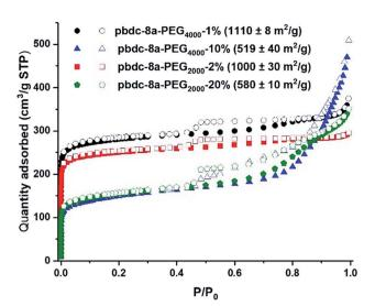
Fig. 6  $N_2$  isotherms of block-polyIRMOF-1 prepared from pbdc-8a-PEG<sub>M<sub>n</sub></sub>-x% polymers.
