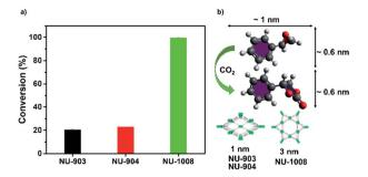
Fig. 6  $CO_2$  fixation conversion on NU-903, NU-904 and NU-1008. (a) Catalytic capacities; (b) size of substrate, product and pore size of NU-903, NU-904 and NU-1008.
