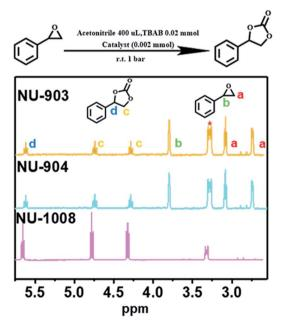
Fig. 5 Proton NMR spectra of  $CO_2$  fixation into styrene oxide catalyzed by NU-903, NU-904 and NU-1008 (1 bar, room temperature, 24 h; CDCl<sub>3</sub> as deuterium solvent, 500 MHz. The peak with asterisk refers to the tetrabutylammonium bromide).
