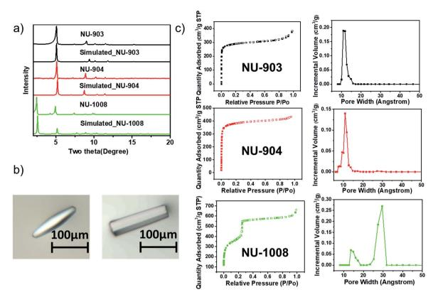
Fig. 3 Characterization of the three MOFs. (a) PXRD patterns; (b) optical images of the single crystals of NU-904 (left) and NU-1008 (right), the scale bars in the images are 100  $\mu$ m; (c) N<sub>2</sub> sorption isotherms and DFT pore size distribution of NU-903, NU-904 and NU-1008.
