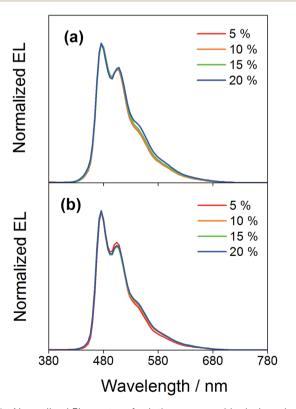
Fig. 6 Normalized EL spectra of solution-processable devices doped with 4 and 7 at different concentrations.
