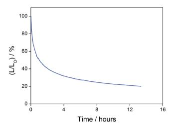
Fig. 10 Relative luminance of vacuum-deposited OLEDs based on 5 wt% complex 7 as a function of operation time at a constant driving current density of 20 mA cm<sup>-2</sup>
