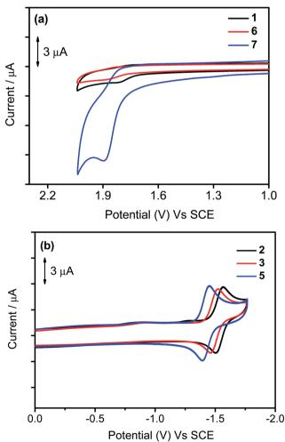
Fig. 5 Cyclic voltammograms for the (a) oxidation of 1, 6, and 7 and (b) reduction scans of 2, 3, and 5 in dichloromethane (0.1 M  $^n$ Bu<sub>4</sub>NPF<sub>6</sub>).
