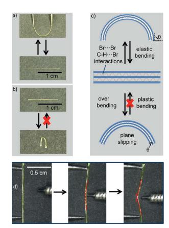
Fig. 4 Photographs of elastic bending (a) and plastic bending (b) under mechanical stress applied through a pair of tweezers; schematic of the crystal before and after elastic or plastic bending (c); and photographs of the overbending process (d).
