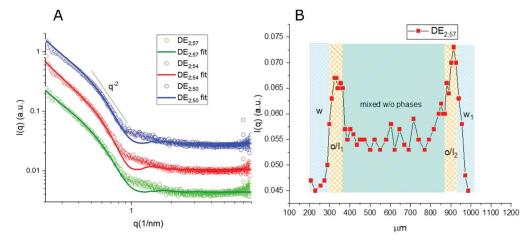
Fig. 3 (A) 1D  $\mu$ -SAXS profile of the w/o/w double emulsion (DE<sub>2</sub>) interface as obtained at the exit of the microfluidic device (RT; green), after storage at 50 °C for 120 min (red) and for 240 min (blue) respectively, (B) SAXS intensity at  $q=0.9~\mathrm{nm}^{-1}$  recorded along an axial line covering a whole DE<sub>2</sub> double emulsion unit.
