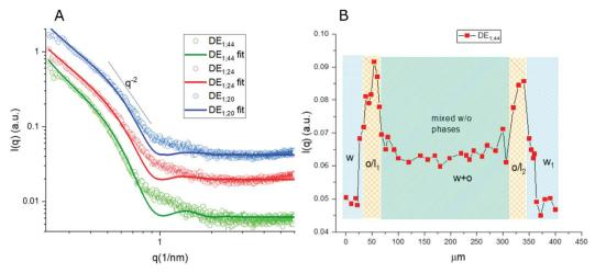
Fig. 2 (A) 1D  $\mu$ -SAXS profile of the w/o/w double emulsion (DE<sub>1</sub>) interface as obtained at the exit of the microfluidic device (RT; green), after storage at 50 °C for 30 min (red) and for 60 min (blue) respectively, (B) SAXS intensity at q=0.74 nm<sup>-1</sup> recorded along an axial line covering a whole DE<sub>1</sub> double emulsion unit. This q value was chosen to minimize the contribution of single bilayers to the overall scattering intensity.
