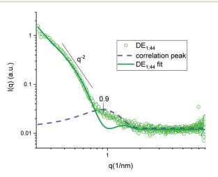
Fig. 4 SAXS intensity of sample DE<sub>1</sub> stored at room temperature fitted by a polydisperse bilayer model (green), with Gaussian peak (violet) superposition to account for inter-bilayer correlation.
