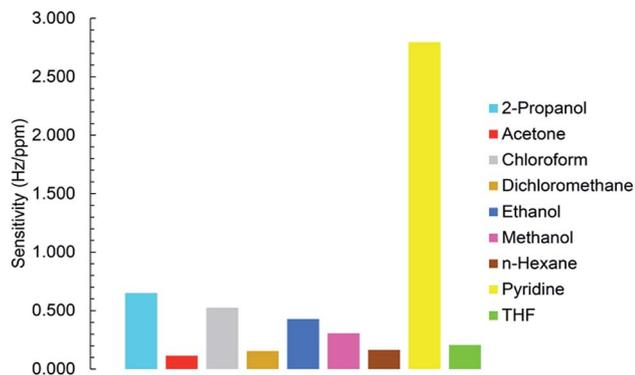
Fig. 11 Sensitivity of sensor to different analytes.
