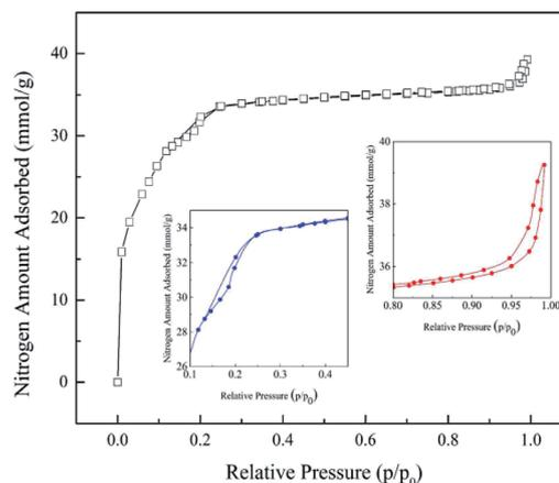
Fig. 5 BET analysis of  $\text{N}_2$  adsorption/desorption in MIL-101(Cr).
