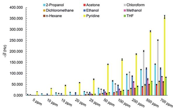
Fig. 8 Sensor responses to different VOCs concentration.
