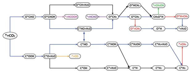
Scheme 1 Most likely reaction pathways for the electroreduction of  $CO_2$  on TM-B<sub>B12</sub>.
