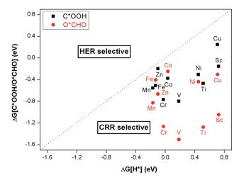
Fig. 3  $\Delta G_{\text{COOH*}}$  and  $\Delta G_{\text{OCHO*}}$  are the Gibbs free energy change of the first protonation step in CRR and  $\Delta G_{H*}$  is for HER. Catalysts below the dotted line are CRR selective.
