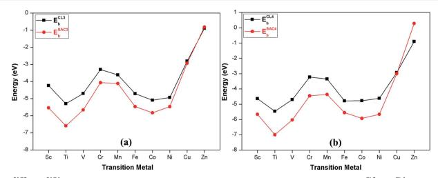
Fig. 2  $E_{\rm b}^{\rm SAC3}$  and  $E_{\rm b}^{\rm SAC4}$  are the binding energies of embedded three and four metal atoms with the B<sub>β12</sub> monolayer.  $E_{\rm b}^{\rm CL3}$  and  $E_{\rm b}^{\rm CL4}$  are the binding energies of metal clusters (comprised of three and four metal atoms) with the  $B_{\rm B12}$  monolayer.
