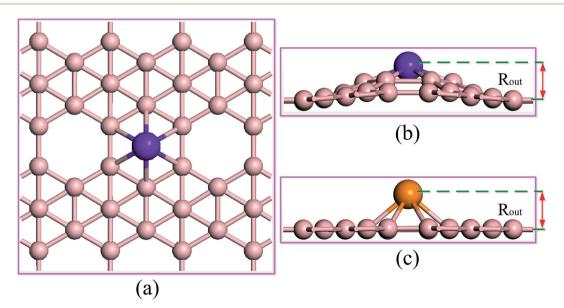
Fig. 1 Optimized geometric structure of the TM-B $_{\beta12}$  monolayers in the 3 imes 3 computational supercell. (a) Top view, (b) and (c) side views. The pastel pink, orange and purple balls represent B, TM (TM = Sc, Cu and Zn) and TM (TM = Ti-Ni), respectively.  $R_{out}$  is the distance between the metal atom and the plane of the  $B_{\beta12}$  sheet.
