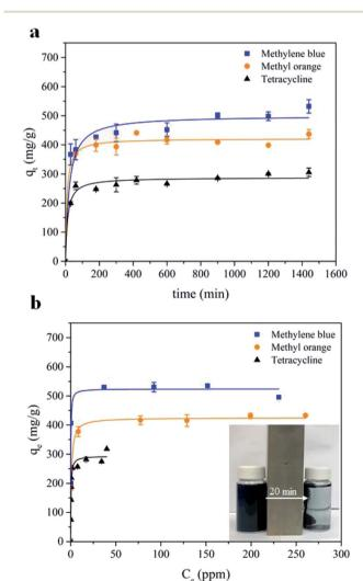
Fig. 3 (a) Adsorption kinetics, and (b) adsorption isotherms of MB, MO and TC adsorption by MWHHTC(1)-800.
