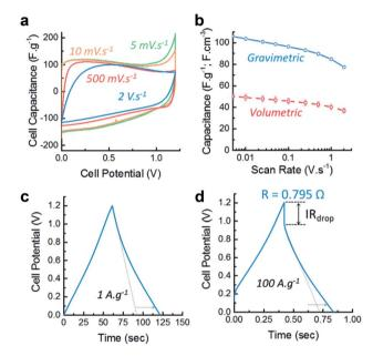
Fig. 5 (a) Cyclovoltammograms (CV) of the symmetric cell at various scan rates; (b) rate capability of the device extracted from the CV curves and corresponding error bars due to the incertitudes on the electrode density measurement; (c) and (d) galvanostatic charge discharge curves at 1 A g $^{-1}$  and 100 A g $^{-1}$  and the corresponding IR $_{\rm drop}$  measurement.
