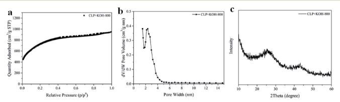
Fig. 4 (a)  $N_2$  sorption-desorption isotherm, (b) pore size distribution calculated by DFT, and (c) XRD pattern of CLP + KOH-800.
