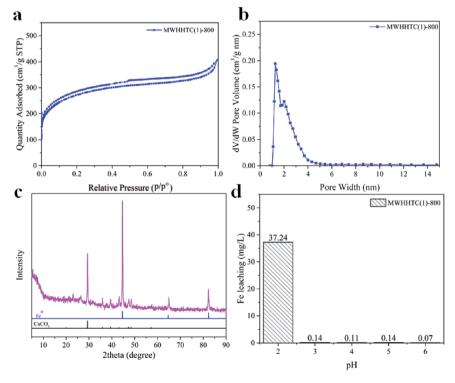
Fig. 1 (a) N<sub>2</sub> sorption-desorption isotherm, (b) pore size distribution calculated by DFT, (c) XRD pattern, and (d) leached iron concentrations at various pHs, for MWHHTC(1)-800
