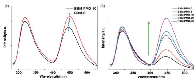
Fig. 5 Fluorescence emission spectra of (a) BBM-Si ( $10^{-6}$  M) and BBM-PMO-10 ( $5 \times 10^{-6}$  g mL<sup>-1</sup>) in THF/H<sub>2</sub>O (3 : 7 v/v); (b) BBM-PMOs in THF/H<sub>2</sub>O (3 : 7 v/v,  $5 \times 10^{-6}$  g mL<sup>-1</sup>), from bottom to top are BBM-PMO-2, BBM-PMO-5, BBM-PMO-10, BBM-PMO-20 and BBM-PMO-40.
