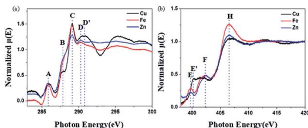
Fig. 8 C (a) and N (b) K-edge XANES spectra of Cu<sup>2+</sup>-chelated BBM-PMO-10, Fe<sup>2+</sup>-chelated BBM-PMO-10 and Zn<sup>2+</sup>-chelated BBM-PMO-10.
