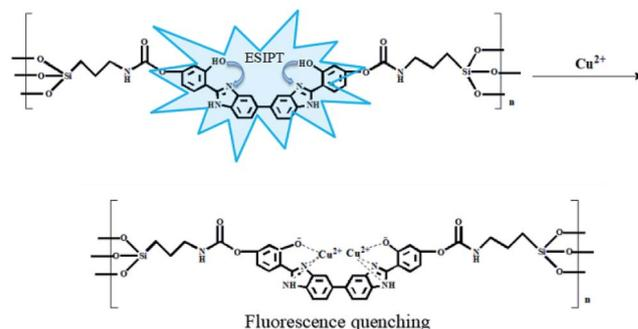
Fig. 9 The mechanism of BBM-PMO detection of Cu<sup>2+</sup>.
