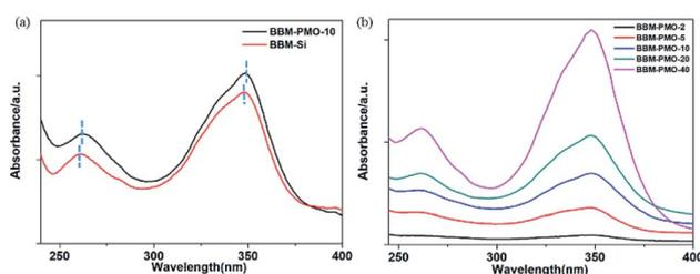
Fig. 4 UV-vis absorption spectra of (a) BBM-Si ( $10^{-5}$  M) and BBM-PMO-10 ( $10^{-4}$  g mL<sup>-1</sup>) in THF/H<sub>2</sub>O (3 : 7 v/v); (b) BBM-PMOs in THF/H<sub>2</sub>O (3 : 7 v/v,  $10^{-4}$  g mL<sup>-1</sup>).
