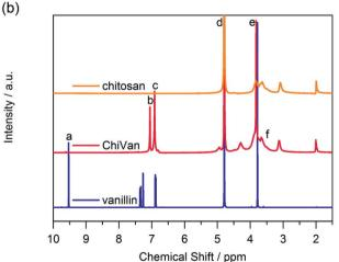
Fig. 1 (a) FT-IR and (b)  $^1\mathrm{H}$  NMR spectra of chitosan, ChiVan, and vanillin in 1% solution of deuterated acetic acid in deuterated water.
