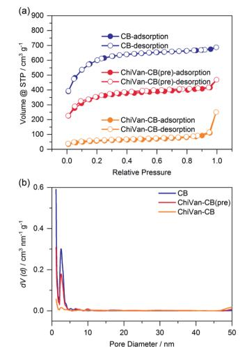
Fig. 2 Nitrogen sorption measurement of carbon black (blue), a ChiVan–CB mixture (red), and ChiVan–CB after grinding (orange). (a) Isotherms and (b) pore size distribution.
