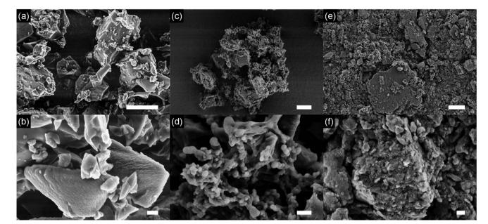
Fig. 3 SEM images of carbon black (a and b) and ChiVan–CB before (c and d) and after (e and f) grinding. The scale bars represent 6 μm (a, c, and e) and 600 nm (b, d, and f), respectively.
