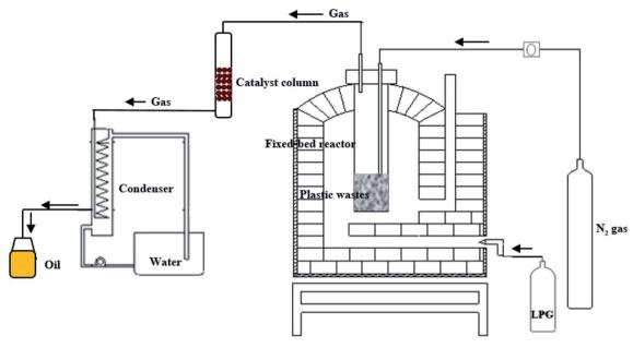
Fig. 1 Schematic diagram of bench scale pyrolysis unit.
