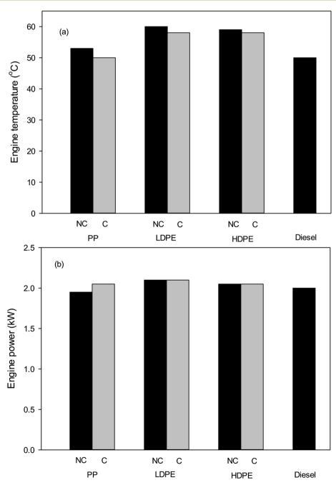
Fig. 7 (a) Engine temperature and (b) power of diesel pump at speed of 2000 rpm (NC = no catalyst and C = catalyst).
