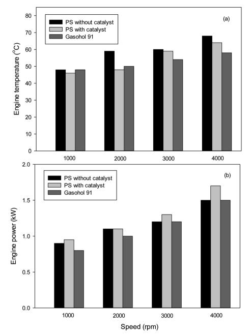
Fig. 6 Variation of engine (a) temperature and (b) power with speed for gasoline brush cutter.
