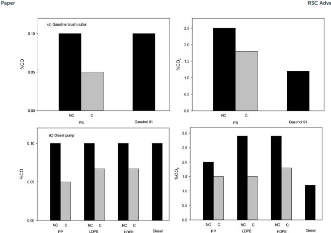
CO and  $CO_2$  emission from (a) gasoline brush cutter and (b) diesel pump at speed of 2000 rpm (NC = no catalyst and C = catalyst)
