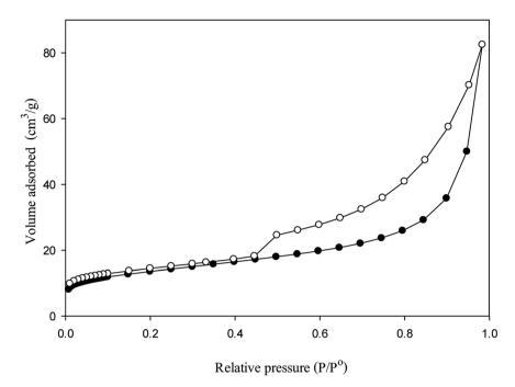
Fig. 3 N<sub>2</sub> adsorption-desorption isotherms at 77 K of bentonite clay.
