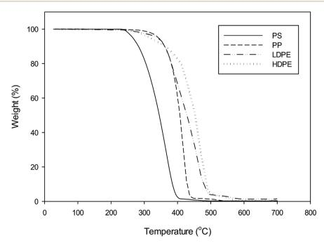
Fig. 2 TGA curves of waste plastics heated under nitrogen at 10 °C min<sup>-1</sup>.
