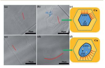
Fig. 3 Optical microscopy images of graphene domains after etching at 1000 °C for (a and b) 10 and (c) 15 min. The gas flow rate of etching was 2:50 (20 sccm  $H_2$  and 500 sccm Ar). (d) Optical microscopy image of GED at 1050 °C. (e and f) Schematics of different etching results between GECRP and GED
