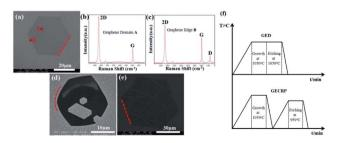
Fig. 1 (a) SEM image of the synthesized hexagonal graphene domain. (b and c) Raman spectra of domain region A and edge B, respectively. (d) SEM image of the graphene domain etched directly after growth. (e) SEM image of the graphene domain etched after cooling and reheating. (f) Simple view of the growth and etching process of the two kinds of samples.
