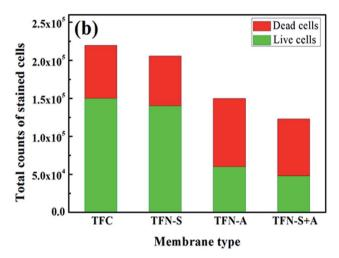
Fig. 5 (a) The biofilm thickness (the error bars represent the standard deviation of three independent measurements); (b) the total counts of stained cells of four fouled membrane.
