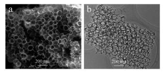
Fig. 5 SEM (a) and TEM (b) images of GS-ALG.
