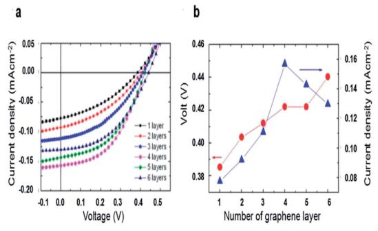
Fig. 5 (a) Current–voltage curves of solar cells based on graphene with 1, 2, 3, 4, 5, and 6 layers under illumination of 730 nm LED (2 mW cm<sup>-2</sup>). (b) The open-circuit voltage and short-circuit current of solar cells measured as functions of the number of graphene layers. (a and b) Reproduced from<sup>51</sup> with permission from American Institute of Physics.
