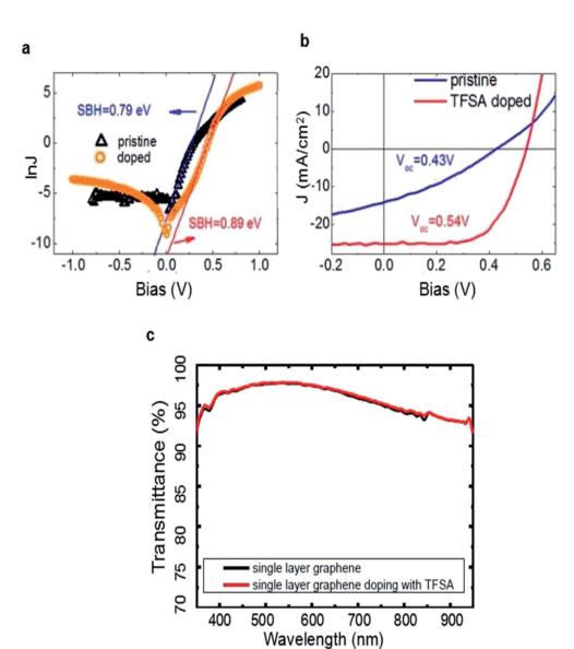
Fig. 3 (a) J-V characteristics in the semi-logarithmic scale. (b) Amplified J-V characteristics of graphene/n-Si diodes. (c) The transmittance spectra of graphene. (a and b) Reproduced from with permission from The American Chemical Society (c) reproduced from with permission from IEEE Xplore.
