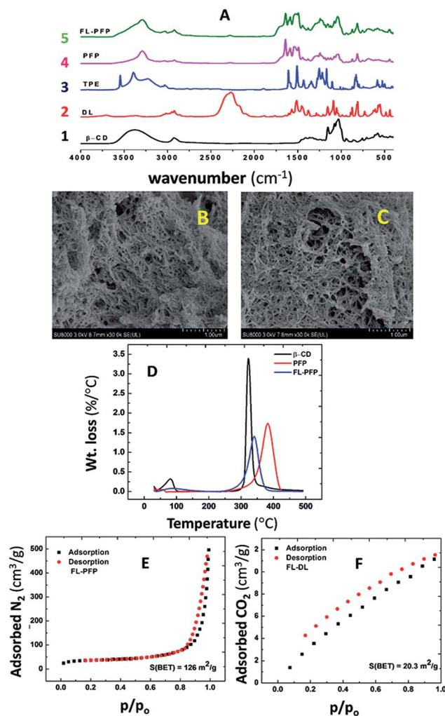
Fig. 1 (A) FT-IR spectra of native  $\beta$ -CD (1), DL (2), TPE (3), PFP (4) and FL-PFP (5), (B) SEM image of PFP, (C) SEM image of FL-PFP, (D) DTA profiles (native  $\beta$ -CD, PFP and FL-PFP) for, (E)  $N_2$  adsorption-desorption isotherm for FL-PFP at  $-196^\circ\text{C}$  and (F)  $\text{CO}_2$  adsorption-desorption isotherm for FL-PFP at  $0^\circ\text{C}$ .
