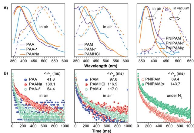
Fig. 4 (A) Emission spectra with  $\tau_0$  of 0 (solid line) and 0.1 ms (dash line) and (B) RTP decay curves of different films (*f*) and powders in air, under nitrogen, or in vacuum. Detailed  $\lambda_{ex}$ s for the emission measurement and monitored wavelengths for the lifetime test are listed in Tables S1 and S2 (ESI<sup>†</sup>).
