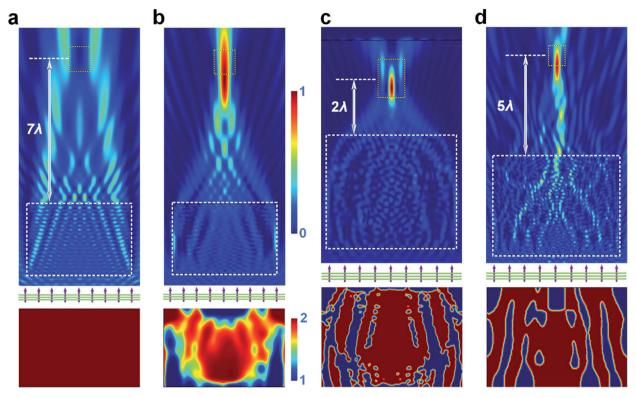
Fig. 6 (a) Scattering by a 2D cuboid without optimization. (b) An elongated PNJ generated by a material layout with index spanning the entire range 1–2. Tight PNJs with (c) short and (d) long focal lengths as generated by binary material layouts with different features.
