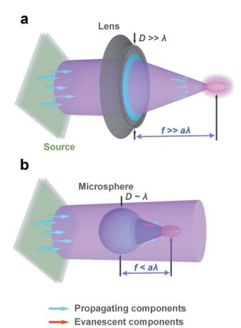
Fig. 1 Schematics of the concentration for the plane-wave excitation based on (a) macroscale and (b) microscale objects. The ideal focal lengths shown in (a) and (b) are far larger and smaller than the wavelength, respectively.
