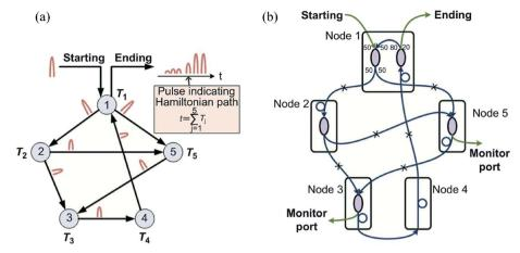
Fig. 15 (a) Schematic of an optical solver for NP-complete problem "Hamiltonian path". (b) Actual design of the network with optical fiber components. This figure has been adapted from ref. 121 with permission from *Light: Science & Applications*.
