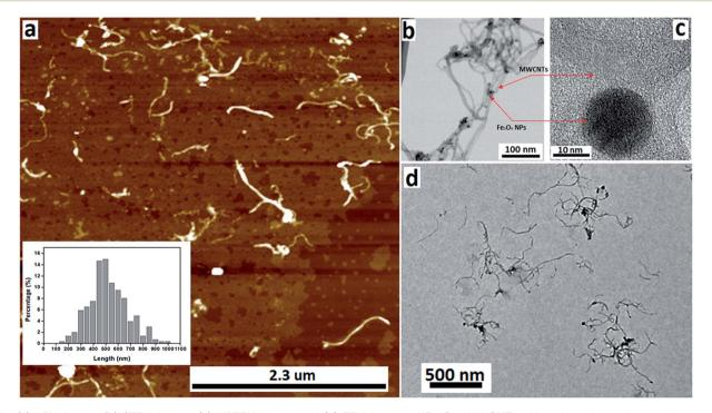
Fig. 3 (a) AFM image, (b) STEM image, (c) HRTEM image and (d) TEM image of  $Fe_3O_4@MWCNT$  exiting the tube under continuous flow (collected), processed in the VFD (optimised parameters) operating at 8.5k rpm rotational speed, with the concentration of the as received MWCNTs at 0.08 mg mL<sup>-1</sup> (DMF), tilt angle 45°, flow rate 0.45 mL min<sup>-1</sup>, and laser power 250 mJ. The inset in (a) is the length distribution of the carbon nanotubes in  $Fe_3O_4@MWCNTs$  (collected).
