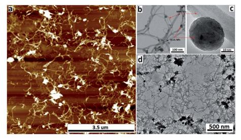
Fig. 2 (a) AFM image, (b) STEM image, (c) HRTEM image and (d) TEM of  $Fe_3O_4@MWCNT$  (retained), formed in the VFD (optimised parameters) operating at 8.5k rpm rotational speed, under continuous flow, with the concentration of the as received MWCNTs at 0.08 mg mL<sup>-1</sup> (DMF), tilt angle 45°, flow rate 0.45 mL min<sup>-1</sup>, and laser power 250 mJ, with the MWCNTs *ca.* 2  $\mu$ m in length.
