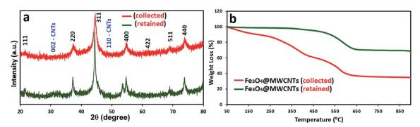
Fig. 5 (a) XRD patterns and (b) TGA curves for  $Fe_3O_4@MWCNT$  exiting (red) and retained (green) in the quartz tube, processed in the VFD (optimised parameters) operating at 8.5k rpm rotational speed, with the concentration of the as received MWCNTs at 0.08 mg mL<sup>-1</sup> (DMF), tilt angle 45°, flow rate 0.45 mL min<sup>-1</sup>, and laser power 250 mJ.
