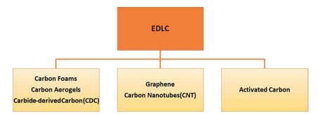
Fig. 2 Classification of electrochemical double layer capacitors (EDLCs)
