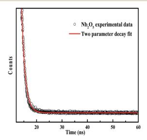
Fig. 6 TRF decay curve of Nb<sub>2</sub>O<sub>5</sub>.
