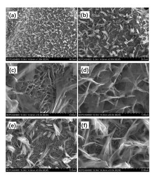
Fig. 4 SEM images of dual-morphology  $ZnCo_2O_4$  on NF (a and b),  $ZnCo_2O_4$  nanosheet (c and d) and feather-like  $ZnCo_2O_4$  (e and f).
