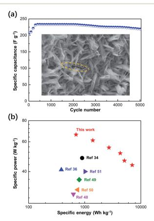
Fig. 9 (a) Cycle life and SEM images of the assembled ZNGN//AC device for 5000 cycles, (b) Ragone plot of the device assembled using the dual-morphology ZnCo<sub>2</sub>O<sub>4</sub> when compared with the recently reported values in the literature. The crack produced after 5000 cycles is highlighted by the yellow dotted circle in (a).
