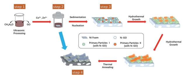
Fig. 6 Schematic of the fabrication process of the 3D hierarchical dual-morphology ZnCo<sub>2</sub>O<sub>4</sub> on NF.
