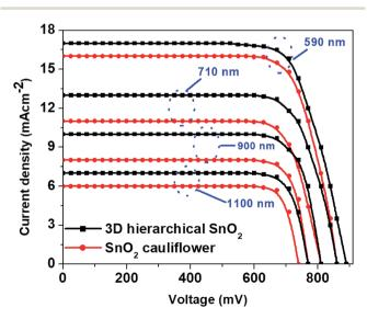
Fig. 3  $\ J-V$  curves as a function of the ETL thickness for two distinct  ${\rm SnO_2}$  nanostructures.
