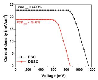
Fig. 7 Comparison of J-V curves of best performing devices of both PSCs and DSSCs based on the 3D hierarchical SnO<sub>2</sub> nanosphere ETL.
