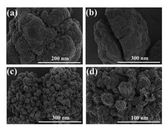
Fig. 1 Plane-view FESEM images of cauliflower-shaped SnO<sub>2</sub> nanospheres at (a) high resolution and (b) low resolution showing that the inside of each cauliflower is made of tiny nanorods and surface FESEM images of 3D hierarchical SnO<sub>2</sub> nanostructures at (c) low resolution and (d) high resolution exhibiting that nanorods are grown over the entire surface of the nanosphere, respectively.
