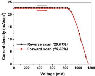
Fig. 5 J-V plot (both in reverse and forward scans) for the best performing PSCs with 3D hierarchical SnO2 nanospheres showing their hysteresis-free behavior.
