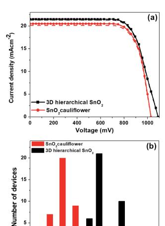
Fig. 2 (a) Comparison of J-V curves of PSCs based on two distinct SnO<sub>2</sub> nanostructures and (b) histograms of the corresponding PSCs showing variations in the PCE for 45 individual cells for each nanostructure.
