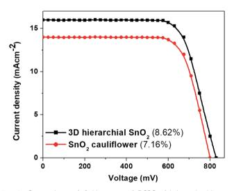
Fig. 6 Comparison of J-V curves of DSSCs fabricated with two distinct SnO<sub>2</sub> nanostructures.
