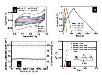
Fig. 5 (a) CV curves for the NVL@CC//AC HSC at various scan rates; (b) GCD curves for the NVL@CC//AC HSC at various current densities; (c) variation of specific capacitance and coulombic efficiency with the number of charge–discharge cycles; (d) EIS spectra for the NVL@CC//AC HSC.
