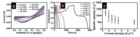
Fig. 3 (a) CV curves for NVL@CC at various scan rates; (b) GCD curves for NVL@CC at various current densities; (c) variation of specific capacity with current density.
