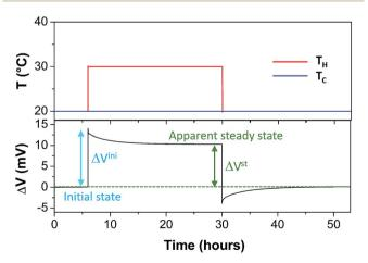
Fig. 2 Typical thermoelectric measurement.  $T_{\rm H}$  is the hot electrode temperature and  $T_{\rm c}$ , the cold electrode temperature. Here, the nanoparticle concentration is 0.28%. An apparent steady state is reached after  $\sim$ 15 hours. See the text for more details.
