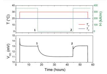
Fig. 8 Variation of apparent steady-state Seebeck voltage in the  $\phi=0.28\%$  sample. The magnetic field is decreased from 360 kA m $^{-1}$  to 0 kA m $^{-1}$  (point 1) and increased again (point 2) while maintaining  $\Delta T=10$  K. The results are reproducible.
