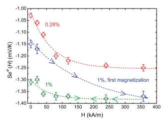
Fig. 6 Apparent steady state Seebeck coefficient as a function of the applied magnetic field (H) for  $\phi=0.28\%$  and  $\phi=1\%$ . The red, blue and green dashed lines are guides to the eye based on the exponential, *i.e.*,  $y=a+be^{\frac{x}{2}}$ .
