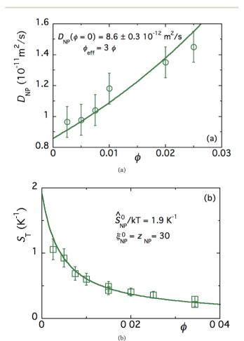
Fig. 3 (a) Diffusion coefficient as a function of NP concentration  $\phi$  of FF-DMSO, measured at room temperature in the absence of a redox couple. The solid line is a fit to eqn (12) as a function of  $\phi$ , without a magnetic field. (b) Soret coefficient measured via the FRS technique as a function of NP concentration ( $\phi$ ), measured at room temperature in the absence of a redox couple. The solid line is a fit to eqn (19) as a function of  $\phi$ , without a magnetic field.
