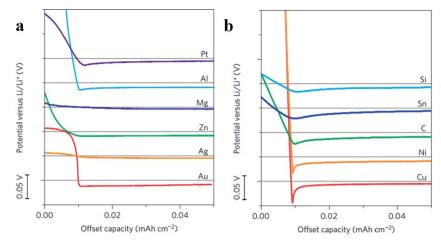
Fig. 15 (a) Voltage profiles of various materials with some solubility in Li during Li deposition at a current density of 10 μA cm<sup>-2</sup>; (b) shifted voltage profiles of various materials with negligible solubility in Li during Li deposition at a current density of 10  $\mu$ A cm<sup>-2</sup>; the horizontal gray lines show 0 V versus Li in (a) and (b). (a-c) Reproduced with permission. <sup>123</sup> Copyright 2016, Nature Publishing Group.
