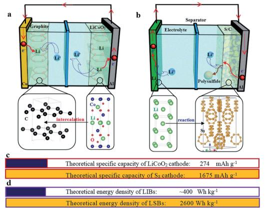
Fig. 2 A schematic illustration of the working principles of a graphite/LiCoO<sub>2</sub> lithium-ion battery (a) and a lithium-sulfur battery (b). The crystal  $structure\ of\ graphite,\ LiCoO_2,\ Li\ metal\ and\ sulfur\ is\ also\ given\ at\ the\ corresponding\ positions.\ (c)\ The\ comparison\ of\ theoretical\ specific\ capacities$ of the LiCoO2 and S8 cathodes. (d) The comparison of theoretical energy densities of LIBs and LSBs.
