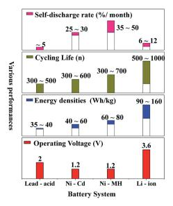
Fig. 1 The performance comparison of various commercialized batteries.
