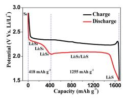
The typical charge-discharge curve of lithium-sulfur batteries.
