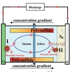
I:  $\text{Li} + S_n^{-2} \rightarrow \text{Li}_2 S \left(\downarrow\right)$ II:  $S_n^{-2} + e^- + \text{Li}^+ \rightarrow \text{Li}_2 S \left(\downarrow\right)$
