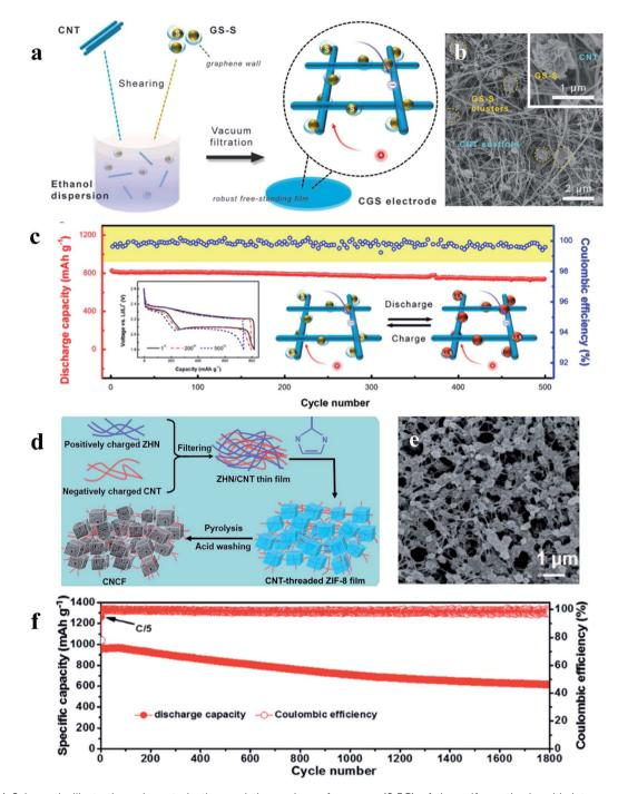
Fig. 8 (a–c) Schematic illustration, characterization and the cycle performance (0.5C) of the sulfur cathode with interconnected carbon nanotube/graphene nanosphere scaffolds; (d–f) schematic illustration, characterization and the cycle performance (1C) of the sulfur cathode with CNT-threaded nitrogen-doped porous carbon films. (a–c) Reproduced with permission.<sup>71</sup> Copyright 2018, Royal Society of Chemistry; (d–f) reproduced with permission.<sup>72</sup> Copyright 2016, Elsevier.
