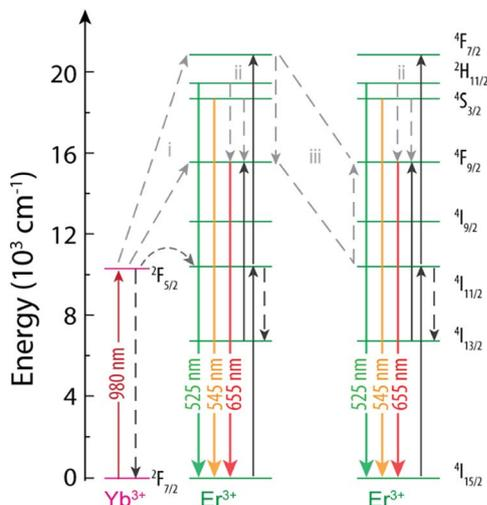
Fig. 5 Partial energy level diagram of  $\text{Yb}^{3+}$  and  $\text{Er}^{3+}$  in  $\text{NaYF}_4:\text{Yb}^{3+}/\text{Er}^{3+}$  NPs.<sup>68</sup> The mechanisms proposed in the literature as being responsible for the variation of the R/G ratio are shown.
