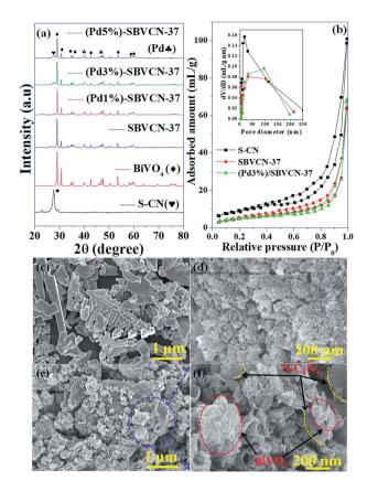
Fig. 1 (a) Powder XRD patterns of all the materials synthesized in this study, (b)  $N_2$  adsorption–desorption isotherms of S-CN, SBVCN-37, and (Pd3%)/SBVCN-37, (inset shows BJH pore size distribution) and FESEM images of (c) BiVO<sub>4</sub>, (d) S-CN, (e) SBVCN-37, and (f) (Pd3%)/SBVCN-37 photocatalyst.
