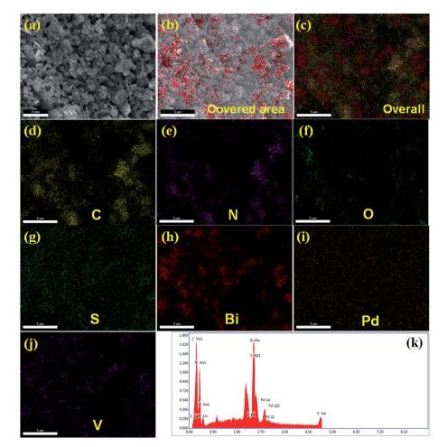
Fig. 2 (a) FESEM image of (Pd3%)/SBVCN-37, (b) covered area for elemental mapping and EDAX, (c) overall mapping, single element mapping of (d) C, (e) N, (f) O, (g) S, (h) Bi, (i) Pd, (j) V, and (k) EDAX spectrum.
