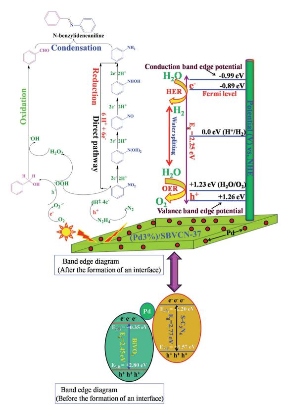
Scheme 1 Proposed mechanism for the photocatalytic one-pot tandem reaction for the synthesis of imine via the reduction of nitrobenzene, oxidation of benzyl alcohol, followed by a condensation reaction and photocatalytic hydrogen evolution reaction (HER) and oxygen evolution reaction (OER) at the surface of the (Pd3%)/SBVCN-37 heterostructure photocatalyst.
