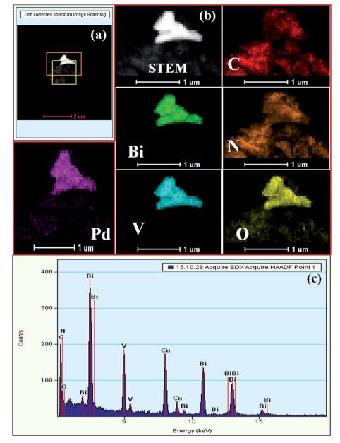
(a) HAADF and (b) STEM-HAADF images of individual elements, and (c) EDAX spectrum of (Pd3%)/SBVCN-37.
