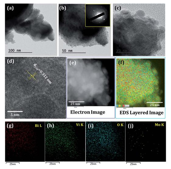
Fig. 5 (a-c) TEM images of Mo:BiVO<sub>4</sub> sample at different magnifications (the inset in b shows the SAED pattern); (d) HRTEM image; (e-j) the corresponding STEM and EDS element mapping images for Bi, V, O and Mo.
