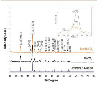
Fig. 3 XRD patterns of bare  $BiVO_4$  and  $Mo:BiVO_4$  thin films synthesized by the ultrasonic spray technique. For comparison, standard diffraction pattern of JCPDS no. 14-0688 is given. The inset shows characteristic peak shift to higher angle  $2\theta$  position.
