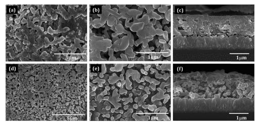
Fig. 2 Scanning electron microscopy images of pristine BiVO<sub>4</sub> (a and b) and Mo:BiVO<sub>4</sub> (d and e) thin films deposited by the ultrasonic technique. (c) Cross-section of BiVO<sub>4</sub> thin film electrodes. (f) Cross-section of Mo:BiVO<sub>4</sub> thin film electrodes (both samples were annealed at 450 °C for 2 h).
