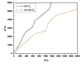
Fig. 8 Electrochemical impedance spectroscopy (EIS) of pristine and Mo:BiVO<sub>4</sub> samples under illumination.
