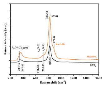
Raman spectra of BiVO<sub>4</sub> and Mo:BiVO<sub>4</sub> nanoporous thin films.
