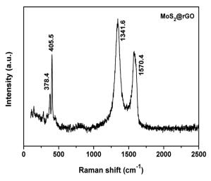
Fig. 2 Raman spectrum of MoS<sub>2</sub>@rGO composite.
