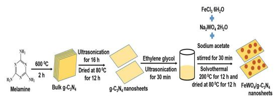
Scheme 1 Schematic representation of the preparation of bulk  $g-C_3N_4$ ,  $g-C_3N_4$  nanosheets and FeWO<sub>4</sub>/ $g-C_3N_4$  nanosheet composites.
