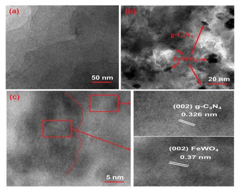
Fig. 3 TEM images of the (a) CNNs and (b) 10-FWO/CNN composite; and (c) HRTEM image of the 10-FWO/CNN composite.
