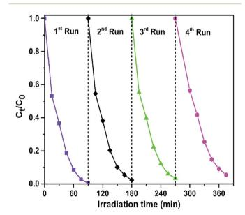
Fig. 9 Recycling photocatalytic tests of the 10-FWO/CNN composite for RhB degradation.
