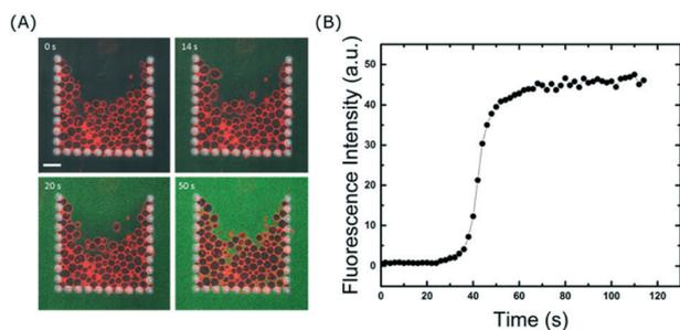
**Fig. 4** Fast and complete fluid exchange. A) Confocal time series of flushing calcein solution into the device at a flow rate of 10  $\mu\text{l min}^{-1}$ . Scale bar: 50  $\mu\text{m}$ . B) Plot of calcein fluorescence taken inside the trap area. Complete solution exchange is achieved after approximately 50 to 60 s.
