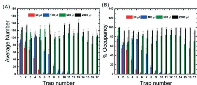
**Fig. 2** Complete filling of device. The average number (A) and % occupancy (B) of GUVs captured in each trap (1 to 17) for increasing volumes flushed in at a flow rate of  $10 \mu\text{L min}^{-1}$ . Vesicle counting is performed manually. Mean values are from three different channels and error bars are taken from the standard deviation of the mean.
