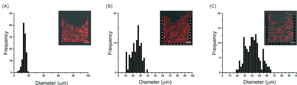
**Fig. 3** Size selection of GUVs. Histograms of trapped GUV diameters for channel heights of (A) 20, (B) 40 and (C)  $60 \mu\text{m}$ . Average diameters were found to be  $14 \pm 1$ ,  $23 \pm 4$ , and  $40 \pm 6 \mu\text{m}$  respectively taken from three separate trap measurements. Inserts: representative fluorescence and bright-field overlays. Scale bars:  $50 \mu\text{m}$ .
