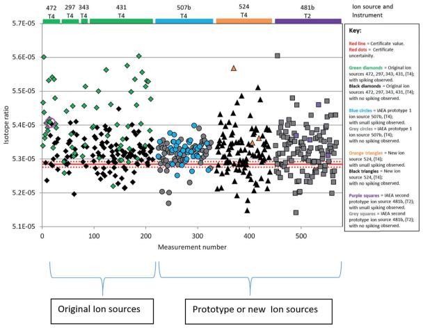
Fig. 9 QC chart displaying total evaporation  $^{234}$ U/ $^{238}$ U data collected on NBL 112-A certified reference material with various ion sources on the IAEA TIMS Triton Plus 'T4' and Triton 'T2'. Pink circled measurement discussed in Fig. 3.
