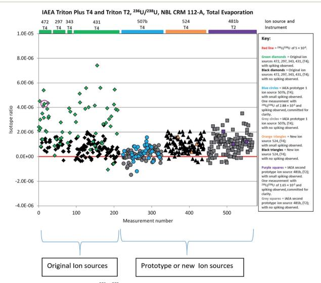
Fig. 10 QC chart displaying total evaporation  $^{236}$ U/ $^{238}$ U data collected on NBL 112-A certified reference material with various ion sources on the IAEA TIMS Triton Plus 'T4' and Triton 'T2'. Pink circled measurement discussed in Fig. 3.
