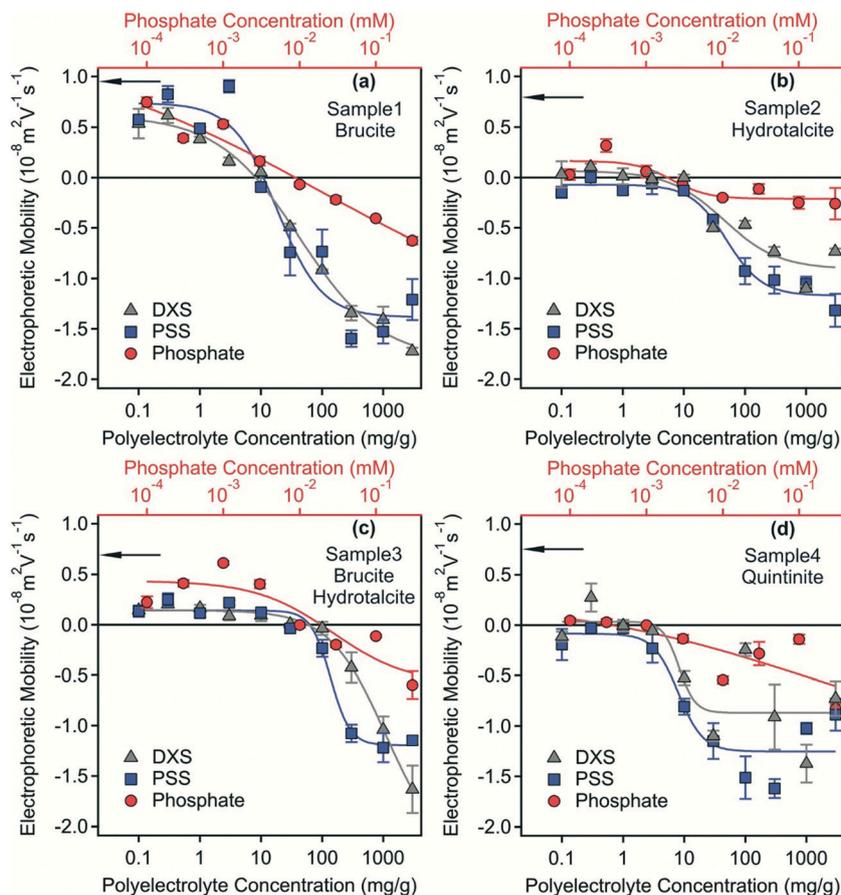
**Fig. 3** Electrophoretic mobilities of particles dispersed in samples 1–4 ((a) sample 1, (b) sample 2, (c) sample 3 and (d) sample 4) as a function of the polyelectrolyte (PSS and DXS) and phosphate concentration. An ionic strength of 80 mM was kept constant in the experiments. The solid lines are for guidance. Arrows indicate the mobilities of the particles prior to flocculants addition.
