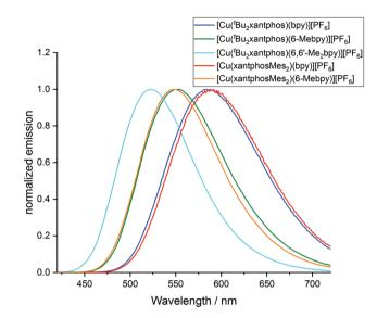
Fig. 12 Normalized solid-state emission spectra of [Cu(P^P)(N^N)][PF<sub>6</sub>] complexes ( $\lambda_{exc}$  = 365 nm).
