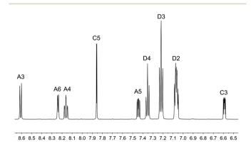
Fig. 4 Aromatic region of the <sup>1</sup>H NMR spectrum (500 MHz, acetone $d_6$ ) of [Cu( ${}^t$ Bu<sub>2</sub>xantphos)(bpy)][PF<sub>6</sub>]. See Fig. S15† for the full spectrum. See Scheme 3 for atom labelling.
