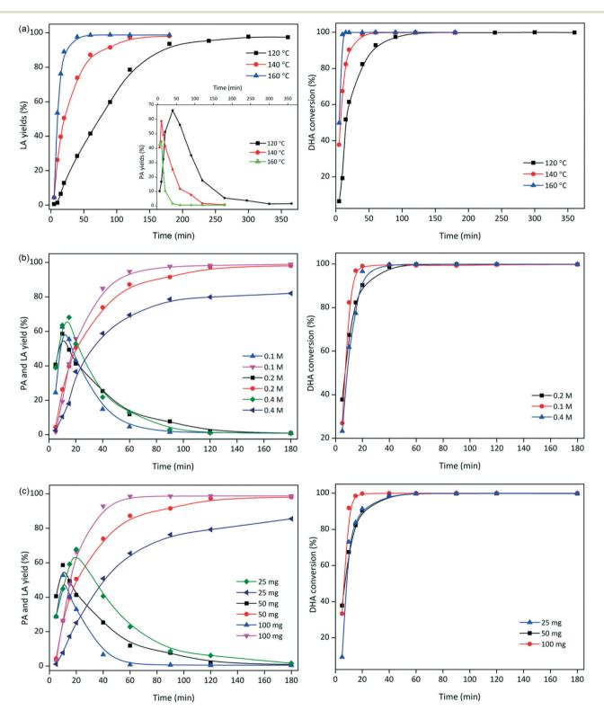
Fig. 6 Optimization of the reaction conditions: (a) reaction temperature, (b) substrate concentration, and (c) catalyst loading (conditions: [DHA]<sub>o</sub> =  $0.2 \text{ M}, \text{SnO}_2/\text{Nb}_2\text{O}_5-3.07 = 50 \text{ mg}, 140 \text{ °C}).$
