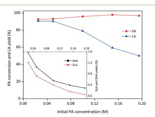
Fig. 7 Effect of the initial PA concentration on the conversion of PA to LA catalyzed by SnO<sub>2</sub>/Nb<sub>2</sub>O<sub>5</sub>-3.07 (conditions: catalyst = 50 mg, 140 °C, 1 h).
