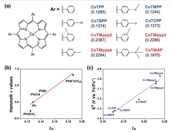
Fig. 3 (a) The chemical structures of functionalized cobalt porphyrins and the corresponding Mulliken charge population on a probe hydrogen atom  $(\chi_H)$  for the aromatic substituents (Ar) shown in parenthesis. (b) Correlation between calculated  $\chi_H$  and the corresponding para position Hammett substituent constant. 30 (c) Correlation between calculated  $\chi_{\rm H}$  and experimentally measured Co(1/11) redox potentials.
