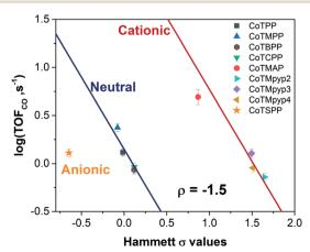
4 TOF<sub>CO</sub> of cobalt porphyrin derivatives with various functionalities versus calculated Hammett  $\sigma$  values (potential: -0.6 V vs. RHE, loading:  $8 \times 10^{-10}$  mol cm<sup>-2</sup>).
