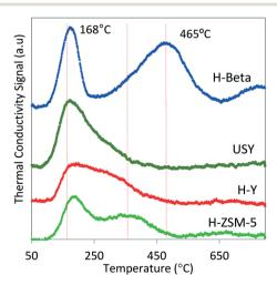
Fig. 2 TPD profiles of ammonia chemisorbed at 100 °C on 60 mg of zeolite. The TPD profiles illustrate the integrated area (decreasing from top to bottom) were normalized to the total surface area and presented as total surface acid capacity (mmol g-1) data shown in Table 2
