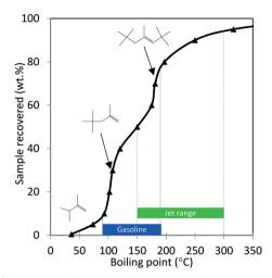
Fig. 9 Simulated distillation profile for the oligomerization product shown in Table 4 collected after 350 hours TOS (Amberlyst-36 catalyst; p = 1.38 MPa, 140 °C, WHSV = 1.1 h<sup>-1</sup>). Proposed structures of major products with corresponding boiling points were obtained from GC-MS analysis.
