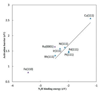
Fig. 3 Activation barriers for N<sub>2</sub> to N<sub>2</sub>H\* reduction on late transition metal surfaces at 0 V-RHE, plotted against N<sub>2</sub>H\* binding energy to the same surface. Blue - FCC(111) metal surfaces, purple - Fe(110) and Ru(0001) surfaces. Linear best fit are shown for FCC metals,  $Ga_1 = 0.93$  $(N_2H \text{ binding energy}) + 3.55 \text{ eV } (R^2 = 0.83).$
