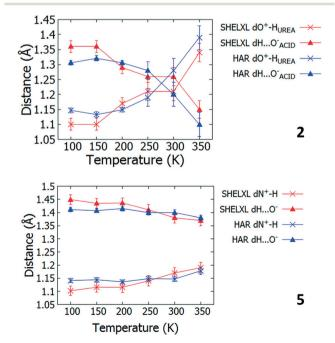
Fig. 4 The D-H and H···A distances in 2 and 5 as refined using SHELXL<sup>57</sup> and HAR<sup>27</sup> over the 100 to 350 K temperature range.
