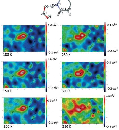
Fig. 11 Fourier difference electron density maps showing the electron density associated with the H-atom in the N<sup>+</sup>-H···O<sup>-</sup> SSHB in 7 over the 100 to 350 K temperature range.
