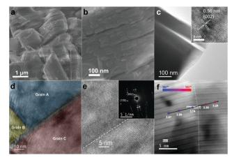
Fig. 3 (a) and (b) SEM images and (c) TEM image of the nanostructured  $P2-Na_{2/3}MnO_2$  (Inset: Magnified HRTEM image). HRTEM images of (d) three neighboring grains: A, B, and C (e) the interface region with a SAED pattern (inset) indicating the different orientations. (f) High-angle annular dark-field STEM image of the interface region with an EELS line scan.
