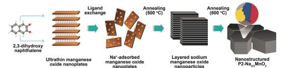
Fig. 1 Schematic illustration of the two-step method to synthesize nanostructured P2-Na<sub>2/3</sub>MnO<sub>2</sub>.
