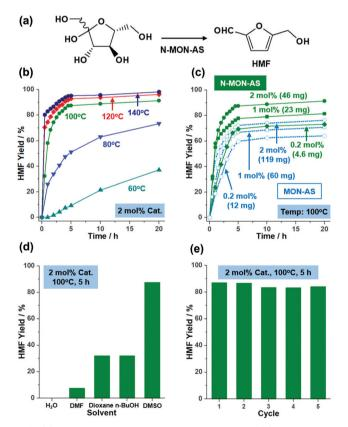
Fig. 4 (a) A scheme of fructose conversion to HMF. (b) Temperature-dependent catalytic performance of N-MON-AS. (c) Comparison of the catalytic performance of MON-AS (0.284 mmol  $SO_3H$  per g) and N-MON-AS (0.731 mmol  $SO_3H$  per g). (d) Solvent-dependent catalytic performance and (e) recyclability of N-MON-AS.
